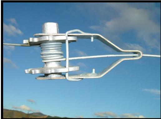
**The Conventional method** is to tie off 1 wire through strap aperture. Then pre-bend point of other end to fit in full depth of spool axle. Leave enough wire slack to allow at least two wraps around spool, before full tension is achieved.
